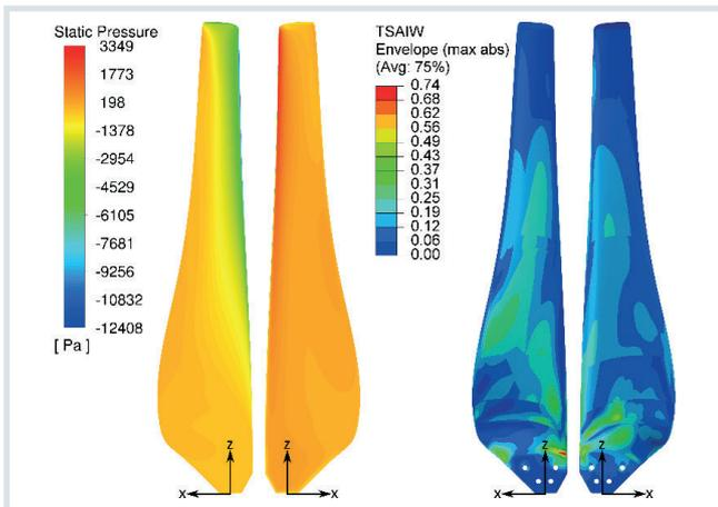
**Fig. 2.** Distribution of pressure on the rotor blade and Tsai-Wu failure criterion (TSAIW). There is no damage to the laminate at TSAIW < 1 © BTU
