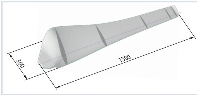
**Fig. 1.** Production-ready implementation of a rotor blade design with the profiles and the profile chord © BTU
