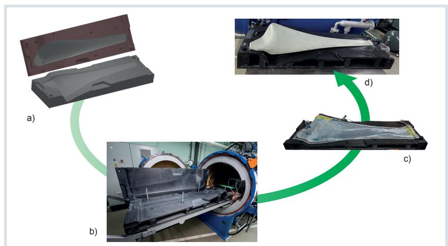
**Fig. 4.** Development of the mold for manufacturing rotor blades. a) CAD model of the mold; b) printed mold; c) infusion of a rotor blade half; d) rotor blade following gluing of both shell halves Source: BTU; graphic: © Hanser
