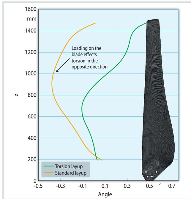
**Fig. 3.** Regression curves (polynomial, degree 6) of torsion angle over blade length at a wind speed of 20 m/s
